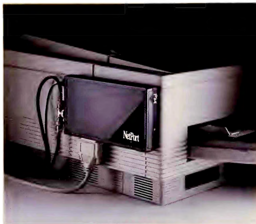
The Intel NetPort is a modem-sized box that lets you connect two printers or plotters directly to your LAN's ethernet cable rather than having to dedicate PCs to the job.
