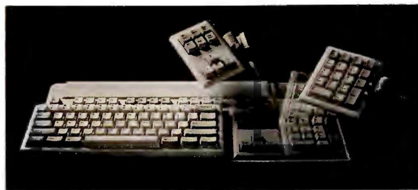
The modular Switchboard lets you customize the locations of keys and add numeric and cursor keypad modules as well as a trackball module that's compatible with the Microsoft Mouse.
