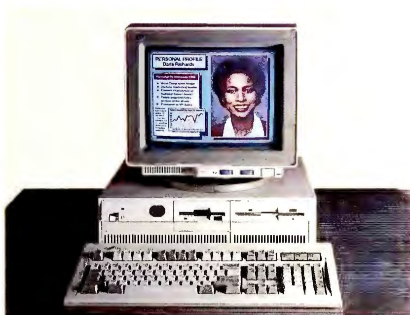
The XGA adapter in IBM's 486 machines runs VGA software faster and displays 1024 by 768 resolution with up to 256 colors.
