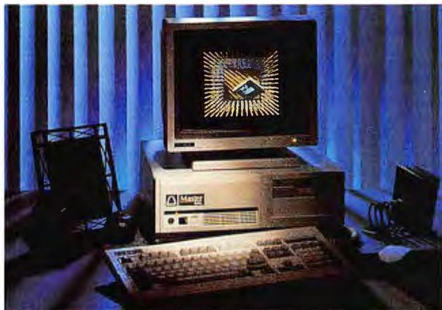
Featuring 4MB of RAM and a 128K memory cache, the Arche Master 486SX-25 is built around Intel's 25-MHz 486SX chip.
