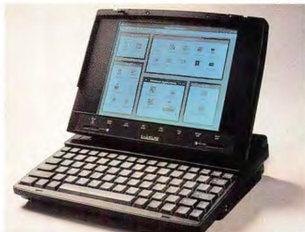
An optional coprocessor encrypts all your files inside the SL007 20-MHz 386SL notebook, which features 4MB of RAM, a 60MB hard drive, and a 10-inch backlit VGA screen.
