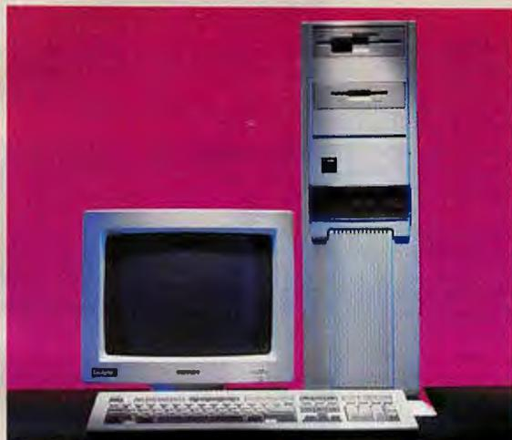
The Insight 20-MHz 486SX includes 4MB RAM, 64K RAM cache, a 130MB IDE hard drive, two floppies, a 14-inch super-VGA monitor, and 16-bit super-VGA card—all for \$1995.
