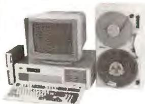
Now you can exchange data files between your IBM PC/XT/AT and any mainframe or mini-computer using IBM compatible 1600 or 6250 BPI 9-Track tape. Unit can also be used for disk backup. Transfer rate is up to 4 megabytes per minute on PCs and compatibles. Subsystems include 7" or 10 1/2" streaming tape drive, tape coupler card, cables and software.
