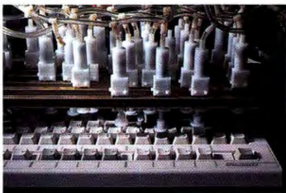
To see how long a keyboard will last, Compaq's robot simulates a lifetime of speed typing.
