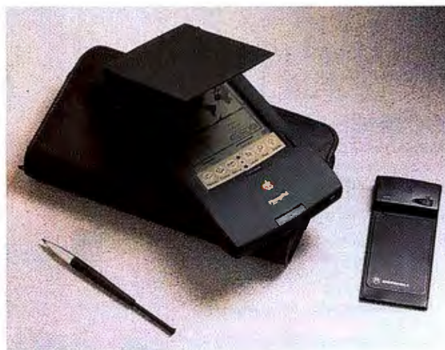
NEWTON'S SECOND CHANCE: Longer and leaner, the new 110 has a flip-up cover, a spring-loaded pen, and a PCMCIA slot on the side.
