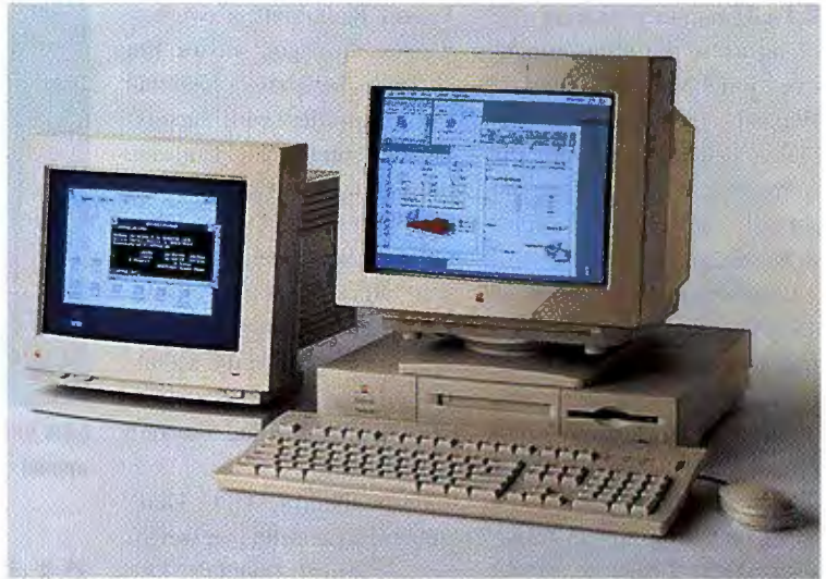
MAC AND PC IN ONE: The Macintosh Quadra 610 features a 486SX-based add-in card that lets it run Mac and Windows/DOS programs simultaneously.
