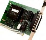
Plug the BuffPort™ into your PC and print to any parallel printer or device. Transfer data from your PC as fast as the printer can accept it, up to 150,000 cps. (A standard PC parallel port is typically limited to about 10,000 cps.) Use the BuffPort with the HWP for a 150,000 cps printer sharing system!
