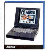
dling most—have a no-slip texture. There's one PCMCIA Type III slot, and RAM upgrades to 20MB. Ambra even builds in sound capabilities. The keyboard is solid and quiet with full-travel action, and the trackball is conveniently positioned front and center.
