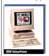
the standard I/O ports. The video setup is excellent, with a 2MB S3based graphics accelerator and a 17-inch monitor supporting flicker-free noninterlaced 75-Hz refresh rates all the way to 1024 by 768 resolution. Nice design touches abound, including a memory upgrade guide and system map pasted to the inside of the case and an available-IRQs list in system setup. The unit pro-
