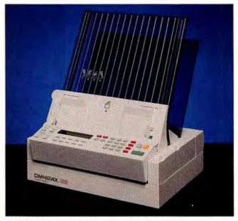
PACKED PERIPHERAL: The Omnifax G5 stuffs a printer, scanner, copier, fax-modem, and fax machine into a 13-pound desktop unit.
