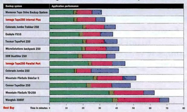
Tape drives are arranged in order of overall performance from best to worst, based on the total of the scores from four equally weighted tests. However, slower performance by a drive in one test may cause its overall bar to be longer than that of a drive with worse overall performance.
