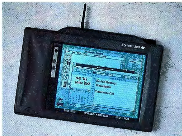
WIRELESS LINK TO THE LAN: Fujitsu's Stylistic RF is a pen-based, hand-held computer that uses a radio signal to connect to a network.
