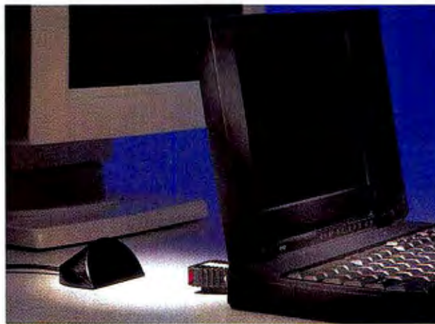
CABLE-FREE FILE TRANSFER: Extended Systems' JetEye uses an infrared signal to transfer data between a notebook and a desktop PC.
