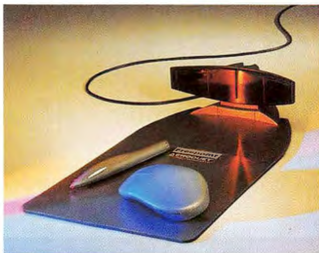
CORDESS MOUSE AND PEN: Creative Labs' AeroDuet uses an infrared link to bring its tangle-free pointers to the desktop.
