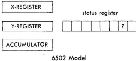
The basic ideas you should be comfortable with at this point are fairly simple. The 6502 microprocessor is our main operational unit. There are three main registers: The accumulator and the X and Y registers. Also present is the status register, which holds a number of one-bit flags to indicate various conditions. So far, the only one we've considered is the Z-flag, for indicating whether a zero or nonzero number is present in one of the other three registers.
